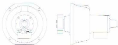
Freno d'emergenza ad arresto progressivo Overspeed safety device with progressive stop
